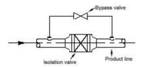
Figure 3 Example for a bypass system
