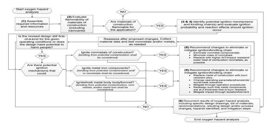
Figure 1 Flowchart showing an oxygen hazard analysis
